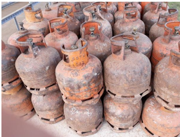
These cylinders are in very poor condition.
